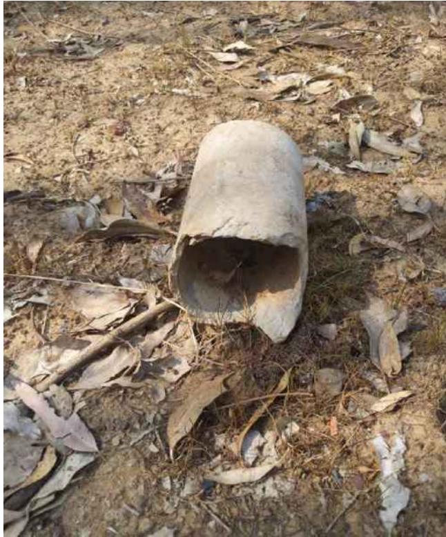
Photo 5 - Potential ACM Pipe
